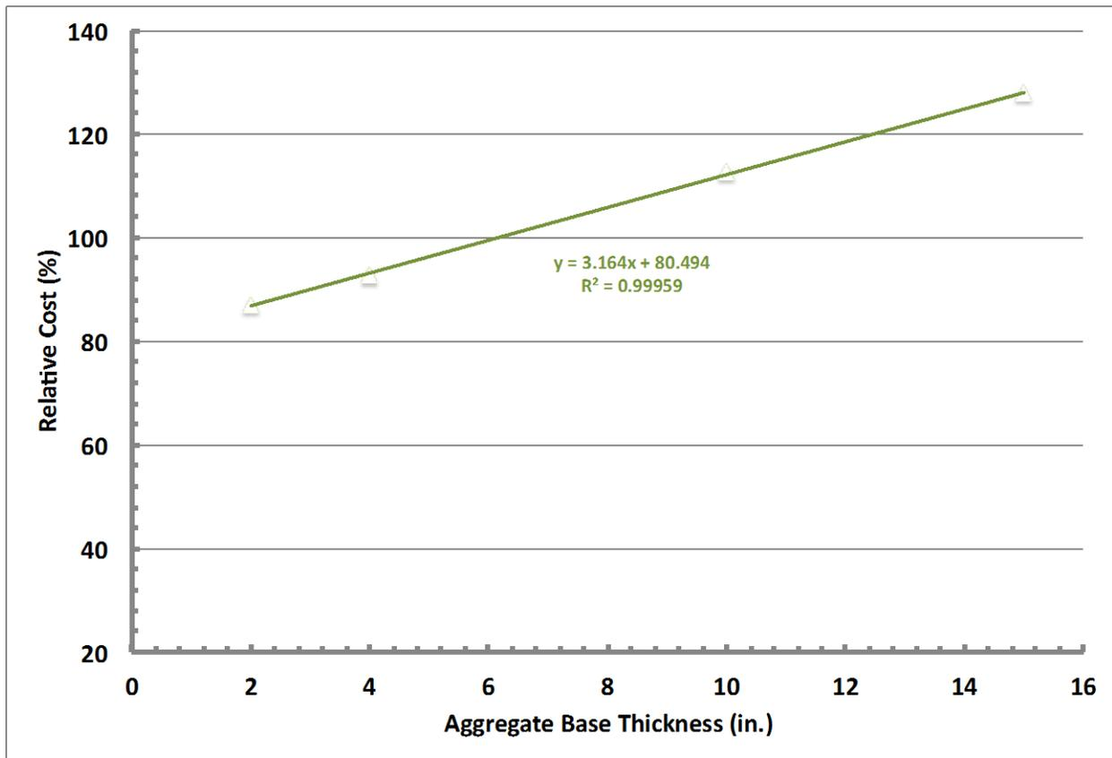
**Figure 6 Aggregate Base Thickness Versus Costs**
