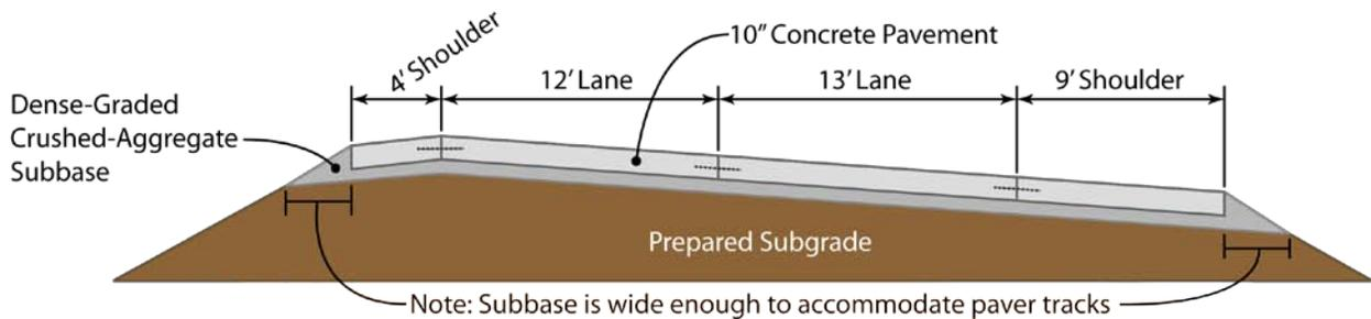
**Figure 2 for Use With Widened Lane Category- Note 13 Dowels in Widened Lane**
