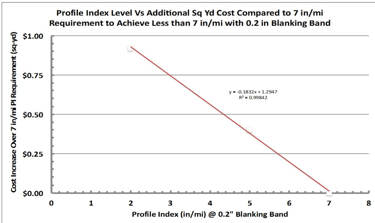
Figure 15 Additional Cost to Achieve the Specified Roughness Compared to Cost to Achieve 7 in./mi. PI with 0.2" Blanking Band
