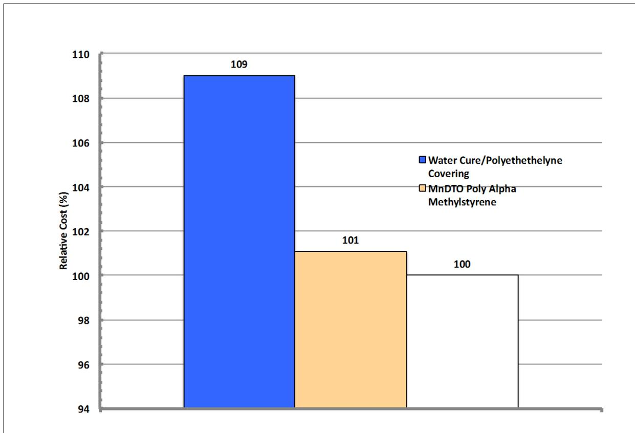
**Figure 10 Survey Results for PCCP Curing Method Options**
