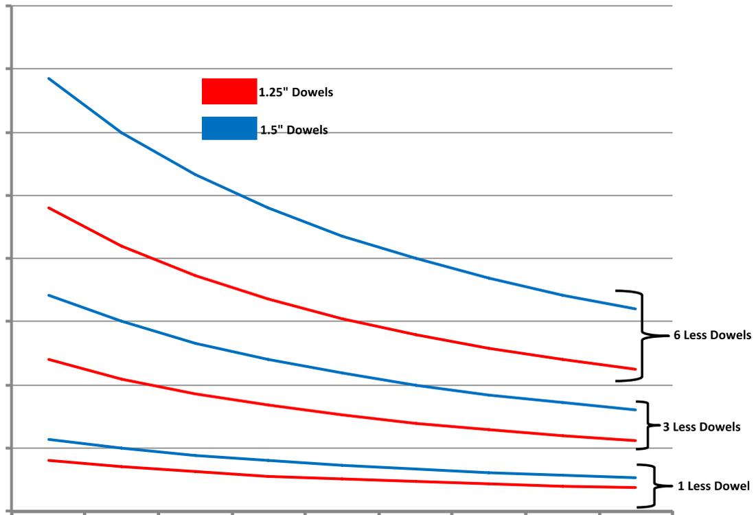
**Figure 16 Change in Cost of Modifying Number of Dowel Bars as a Percentage of the In-Place Cost of the Concrete Pavement (sq. yd.)**
