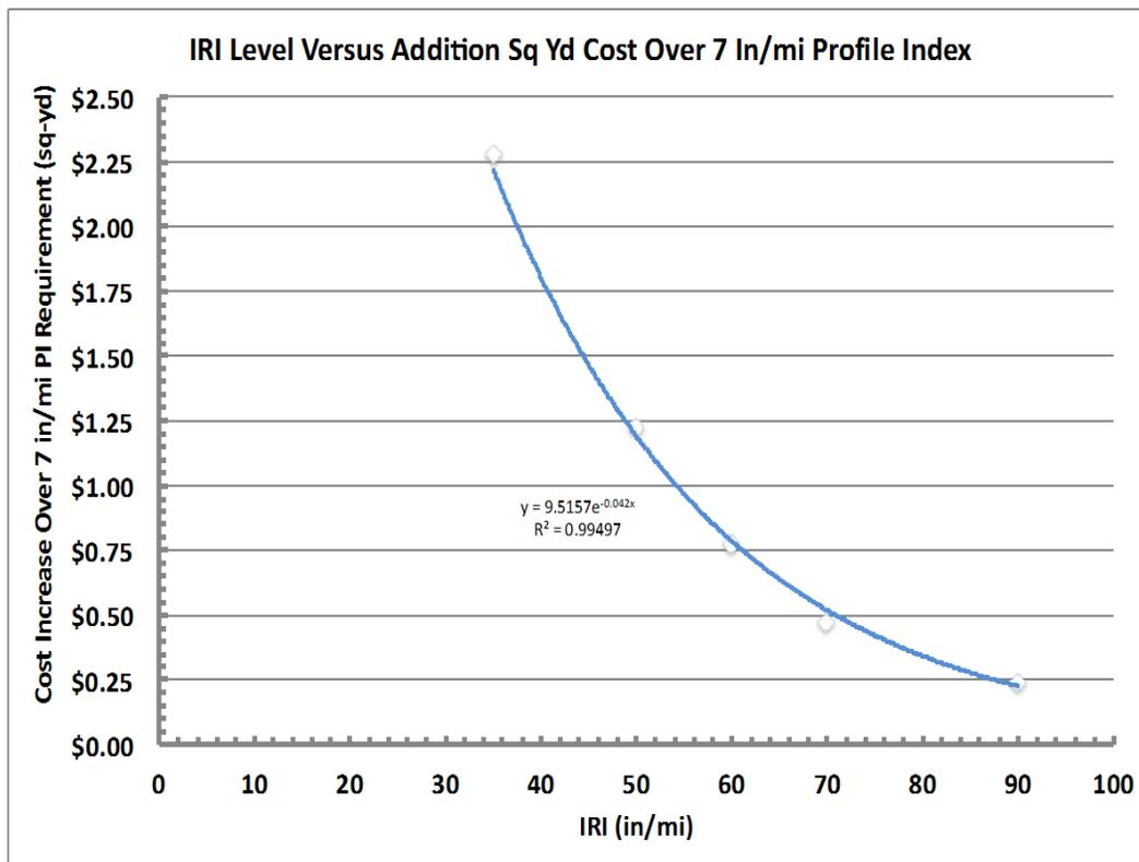
Figure 13 IRI Level Versus Additional Cost to Achieve the Specified Roughness Compared to the Cost to Achieve 7 in./mi. PI with 0.0" Blanking Band
