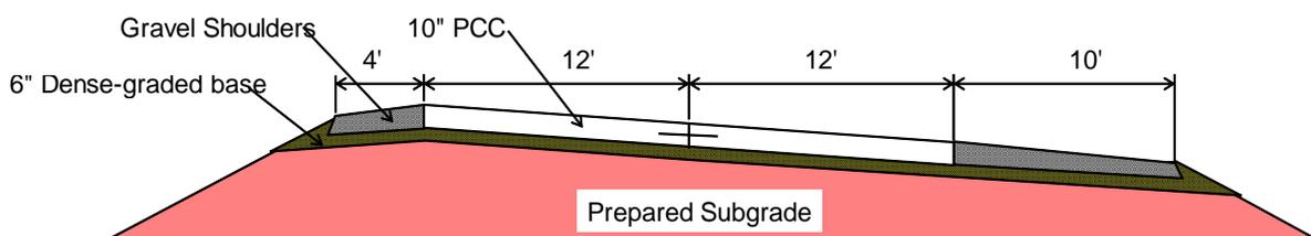
**Figure 1 1995 Standard Reference Section**
